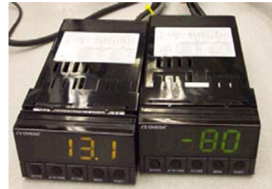
Figure 9. Omega DP25B-S-A Strain Gauge Meter.
