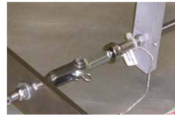
Figure 7. Omega LC-201 Load Cell.
