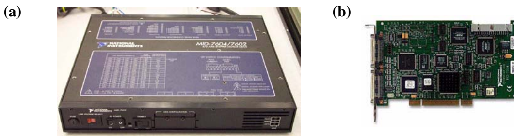
Figure 5. (a) MID-7602 Stepper Motor Drive; (b) PCI-7342 Motion Control Hardware.
